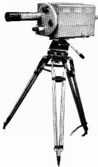
"Pyetron" television camera with rotatable triple-lens turret as used by Pye Ltd. for the demonstration transmissions during the British Exhibition in Copenhagen.
